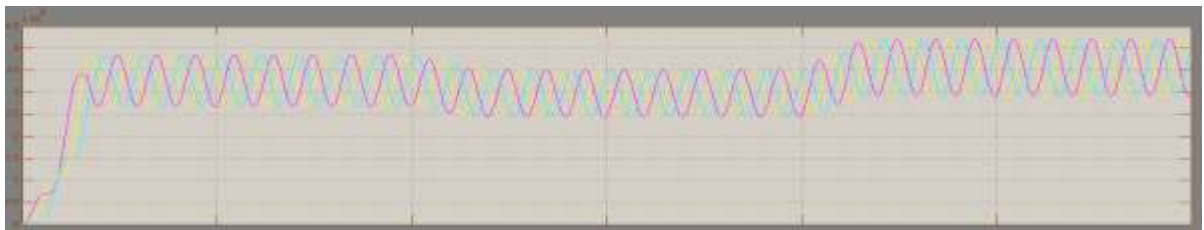
Fig. 9(a) Active and Reactive power waveform with D-STATCOM
